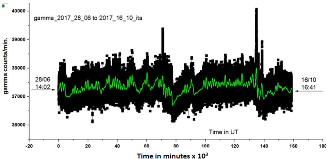
Measurements of gamma rays in the range of 06/28/2017 to 10/16/2017. Green line is smoothed curve of 1day
