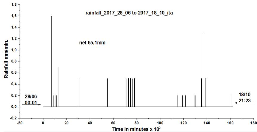
Spectrum in function of the time of the rains occurred every minute between 06/28 to 10/16 of 2017
